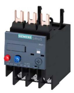
OVERLOAD RELAY 2.2...3.2 A FOR MOTOR PROTECTION SZ S0, CLASS 10, F. MOUNTING ONTO CONTACTOR MAIN CIRCUIT: RING CABLE LUG AUX. CIRCUIT: RING CABLE LUG MANUAL-**AUTOMATIC-RESET**
