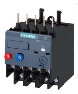
OVERLOAD RELAY 7.0...10 A FOR MOTOR PROTECTION SZ S00, CLASS 10, F. MOUNTING ONTO CONTACTOR MAIN CIRCUIT: RING CABLE LUG AUX. CIRCUIT: RING CABLE LUG MANUAL-AUTOMATIC-RESET
