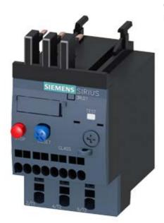
OVERLOAD RELAY 2.2...3.2 A FOR MOTOR PROTECTION SZ S00, CLASS 10, F. MOUNTING ONTO CONTACTOR MAIN CIRCUIT: SPRING TERMINAL AUX. CIRCUIT: SPRING TERMINAL MANUAL-AUTOMATIC-RESET
