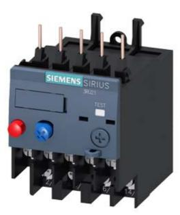
OVERLOAD RELAY 1.1...1.6 A FOR MOTOR PROTECTION SZ S00, CLASS 10, F. MOUNTING ONTO CONTACTOR MAIN CIRCUIT: RING CABLE LUG AUX. CIRCUIT: RING CABLE LUG MANUAL-AUTOMATIC-RESET
