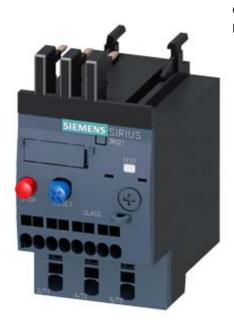
OVERLOAD RELAY 1.1...1.6 A FOR MOTOR PROTECTION SZ S00, CLASS 10, F. MOUNTING ONTO CONTACTOR MAIN CIRCUIT: SPRING TERMINAL AUX. CIRCUIT: SPRING TERMINAL MANUAL-AUTOMATIC-RESET
