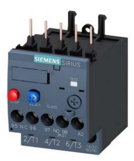
OVERLOAD RELAY 0.45...0.63 A FOR MOTOR PROTECTION SZ S00, CLASS 10, F. MOUNTING ONTO CONTACTOR MAIN CIRCUIT: SCREW TERMINAL AUX. CIRCUIT: SCREW TERMINAL MANUAL-AUTOMATIC-RESET
