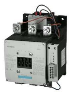
CONTACTOR, 250KW/400V/AC-3 AC(50...60HZ)/DC OPERATION UC 200-277V AUXILIARY CONTACTS 1NO+1NC 3-POLE, SIZE S12 BAR CONNECTIONS ELECTRONIC OPERATING MECHANISM WITH PLC/SIMOCODE INTERFACE AND REMAIN. LIFETIME INDICATOR
