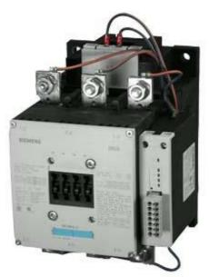
CONTACTOR, 200KW/400V/AC-3 AC(50...60HZ)/DC OPERATION UC 200-277V AUXILIARY CONTACTS 1NO+1NC 3-POLE, SIZE S12 BAR CONNECTIONS ELECTRONIC OPERATING MECHANISM WITH PLC/SIMOCODE INTERFACE AND REMAIN. LIFETIME INDICATOR
