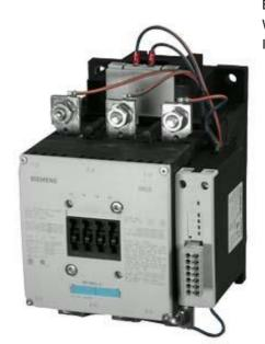
CONTACTOR, 200KW/400V/AC-3 AC(50...60HZ)/DC OPERATION UC 96-127V AUXILIARY CONTACTS 1NO+1NC 3-POLE, SIZE S12 BAR CONNECTIONS ELECTRONIC OPERATING MECHANISM WITH PLC/SIMOCODE INTERFACE AND REMAIN. LIFETIME INDICATOR
