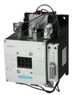
CONTACTOR, 160KW/400V/AC-3 AC(50...60HZ)/DC OPERATION UC 96-127V AUXILIARY CONTACTS 1NO+1NC 3-POLE, SIZE S10 BAR CONNECTIONS ELECTRONIC OPERATING MECHANISM WITH PLC/SIMOCODE INTERFACE AND REMAIN. LIFETIME INDICATOR
