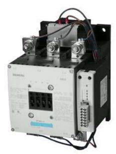
CONTACTOR, 132KW/400V/AC-3 AC(50...60HZ)/DC OPERATION UC 96-127V AUXILIARY CONTACTS 1NO+1NC 3-POLE, SIZE S10 BAR CONNECTIONS ELECTRONIC OPERATING MECHANISM WITH PLC/SIMOCODE INTERFACE AND REMAIN. LIFETIME INDICATOR
