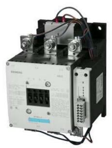
CONTACTOR, 110KW/400V/AC-3 AC(50...60HZ)/DC OPERATION UC 200-277V AUXILIARY CONTACTS 1NO+1NC 3-POLE, SIZE S10 BAR CONNECTIONS ELECTRONIC OPERATING MECHANISM WITH PLC/SIMOCODE INTERFACE AND REMAIN. LIFETIME INDICATOR
