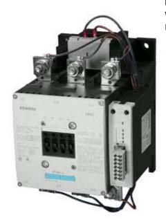
CONTACTOR, 110KW/400V/AC-3 AC(50...60HZ)/DC OPERATION UC 96-127V AUXILIARY CONTACTS 1NO+1NC 3-POLE, SIZE S10 BAR CONNECTIONS ELECTRONIC OPERATING MECHANISM WITH PLC/SIMOCODE INTERFACE AND REMAIN. LIFETIME INDICATOR
