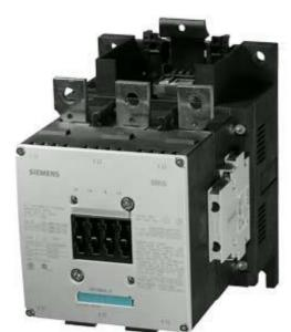
CONTACTOR, 110KW/400V/AC-3 WITHOUT COIL AUXILIARY CONTACTS 2NO+2NC 3-POLE, SIZE S10 BAR CONNECTIONS CONVENT. OPERATING MECHANISM AUX.COND.: SCREW TERMINALS
