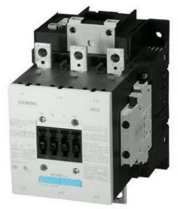
CONTACTOR, 90KW/400V/AC-3, AC(50...60HZ)/DC OPERATION UC 200...277V AUXIL. CONTACTS 2NO+2NC 3-POLE, SIZE S6 BAR CONNECTIONS ELECTRONIC OPERATING MECHANISM WITH 24V DC PLC INTERFACE SCREW TERMINAL
