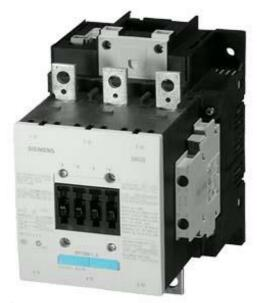
CONTACTOR, 90KW/400V/AC-3, AC(50...60HZ)/DC OPERATION UC 21...27.3V AUXIL. CONTACTS 2NO+2NC 3-POLE, SIZE S6 BAR CONNECTIONS ELECTRONIC OPERATING MECHANISM WITH 24V DC PLC INTERFACE SCREW TERMINAL
