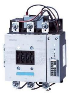
CONTACTOR, 775KW/400V/AC-3, AC(50...60HZ)/DC OPERATION UC 200...277V AUXIL. CONTACTS 1NO+1NC 3-POLE, SIZE S6 BAR CONNECTIONS ELECTRONIC OPERATING MECHANISM WITH PLC/SIMOCODE INTERFACE AND REMAIN. LIFETIME INDICATOR
