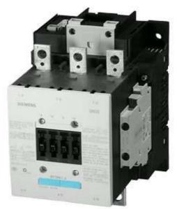
CONTACTOR, 75KW/400V/AC-3, AC(50...60HZ)/DC OPERATION UC 200...277V AUXIL. CONTACTS 2NO+2NC 3-POLE, SIZE S6 BAR CONNECTIONS ELECTRONIC OPERATING MECHANISM WITH PLC INTERFACE 24V DC SCREW TERMINAL
