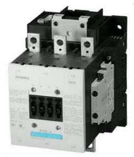
CONTACTOR, 75KW/400V/AC-3, AC(50...60HZ)/DC OPERATION UC 21...27.3V AUXIL. CONTACTS 2NO+2NC 3-POLE, SIZE S6 BAR CONNECTIONS ELECTRONIC OPERATING MECHANISM WITH PLC INTERFACE 24V DC SCREW TERMINAL
