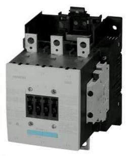
CONTACTOR, 75KW/400V/AC-3 W/O COIL AUXIL. CONTACTS 2NO+2NC 3-POLE, SIZE S6 BAR CONNECTIONS CONVENTIONAL OPERATING MECHAN. AUX. CONDUCTOR: SCREW TEMRINALS
