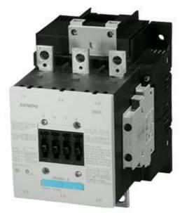
CONTACTOR, 75KW/400V/AC-3, AC(50...60HZ)/DC OPERATION UC 220...240V AUXIL. CONTACTS 2NO+2NC 3-POLE, SIZE S6 BAR CONNECTIONS CONVENTIONAL OPERATING MECHAN. SCREW TERMINAL
