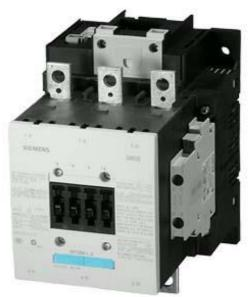
CONTACTOR, 55KW/400V/AC-3 AC(50...60HZ)/DC OPERATION UC 21...27.3V AUXIL. CONTACTS 2NO+2NC 3-POLE, SIZE S6 BAR CONNECTIONS ELECTRONIC OPERATING MECHANISM WITH PLC INTERFACE 24V DC SCREW TERMINAL
