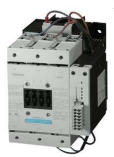
CONTACTOR, 55KW/400V/AC-3 AC(50...60HZ)/DC OPERATION UC 96-127V AUXILIARY CONTACTS 1NO+1NC 3-POLE, SIZE S6 WITH BOX TERMINALS ELECTRONIC OPERATING MECHANISM WITH PLC/SIMOCODE INTERFACE AND REMAIN. LIFETIME INDICATOR
