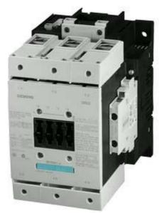
CONTACTOR, 55KW/400V/AC-3 AC(50...60HZ)/DC OPERATION UC 96...127V AUXIL. CONTACTS 2NO+2NC 3-POLE, SIZE S6 WITH BOX TERMINALS ELECTRONIC OPERATING MECHANISM WITH PLC INTERFACE 24V DC SCREW TERMINAL
