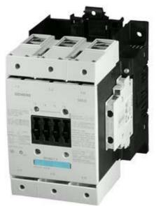
CONTACTOR, 55KW/400V/AC-3 W/O COIL AUXIL. CONTACTS 2NO+2NC 3-POLE, SIZE S6 WITH BOX TERMINALS CONVENTIONAL OPERATING MECHAN. AUX.CONDUCTOR: SCREW TERMINALS
