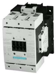
CONTACTOR, 55KW/400V/AC-3 AC(50...60HZ)/DC OPERATION UC 110...127V AUXIL. CONTACTS 2NO+2NC 3-POLE, SIZE S6 WITH BOX TERMINALS CONVENTIONAL OPERATING MECHAN. **SCREW TERMINAL**
