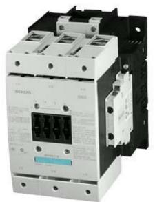
CONTACTOR, 55KW/400V/AC-3 AC(50...60HZ)/DC OPERATION UC 23...26V AUXIL. CONTACTS 2NO+2NC 3-POLE, SIZE S6 WITH BOX TERMINALS CONVENTIONAL OPERATING MECHAN. SCREW TERMINAL
