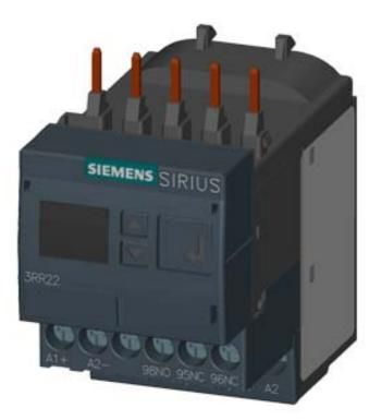
MONITORING RELAY ATTACHABLE TO CONTACTOR 3RT2. SIZE S00 STANDARD, DIGITAL ADJUSTABLE APPARENT/ACTIVE CURRENT MONIT. 1.6 - 16A, 20-400 HZ, 3-PHASE SUPPLY 24-240 V AC/DC 1 CO CONTACT, 1 SEMICOND. FOR ALARM AND WARNING MONITORING FOR CURRENT OVERSHOOT/UNDERSHOOT PHASE FAILURE, WIRE BREAK PHASE SEQUENCE FAULT CURRENT BLOCKING CURRENT WARNING AND ALARM THRESHOLDS WITH OR W/O ERROR LOG ONDELAY 0-99 S SPURIOUS PEAK SUPPR. 0-30 S BREAK AFTER FAULT 0-300 MIN SCREW CONNECTION
