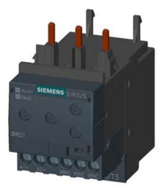
MONITORING RELAY ATTACHABLE TO CONTACTOR 3RT2. SIZE S0 BASIC, ANALOG ADJUSTABLE APPARENT CURRENT MONITORING 4 - 40A, 50-60 HZ, 2-PHASE SUPPLY 24-240 V AC/DC 1 CO CONTACT MONITORING FOR CURRENT OVERSHOOT/UNDERSHOOT PHASE FAILURE, WIRE BREAK WITH OR W/O ERROR LOG ON-DELAY 0-60 S SPURIOUS PEAK SUPPR.0-30 S SWITCHING HYSTERESIS 6% SCREW CONNECTION
