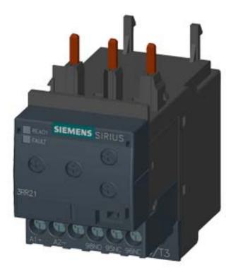
MONITORING RELAY ATTACHABLE TO CONTACTOR 3RT2. SIZE S0 BASIC, ANALOG ADJUSTABLE APPARENT CURRENT MONITORING 4 - 40A, 50-60 HZ, 2-PHASE SUPPLY 24 V AC/DC 1 CO CONTACT MONITORING FOR CURRENT OVERSHOOT/UNDERSHOOT PHASE FAILURE, WIRE BREAK WITH OR W/O ERROR LOG ON-DELAY 0-60 S SPURIOUS PEAK SUPPR.0-30 S SWITCHING HYSTERESIS 6% SCREW CONNECTION
