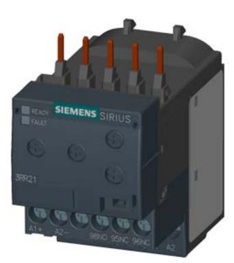
Monitoring relay, attachable to contactor 3RT2, size S00 Basic, analog adjustment Apparent current monitoring 1.6-16 A, 20-400 Hz, 2-phase Supply 24 V AC/DC 1 changeover contact Monitoring for current overshoot and undershoot Phase failure, wire break with or without fault buffer ON delay 0-60 s Spurious peak suppr. 0-30 s Switching hysteresis 6% Screw terminal
