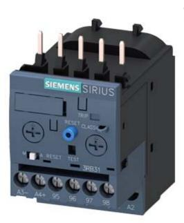
OVERLOAD RELAY 3...12 A FOR MOTOR PROTECTION SIZE S00, CLASS 5...30 CONTACTOR ASS. MAIN CIRCUIT: SCREW CONN. AUX.CIRCUIT: SCREW CONN. MANUAL-AUTOM.-RESET INT. GROUND FAULT DETECTION
