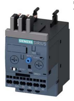
OVERLOAD RELAY 1...4 A FOR MOTOR PROTECTION SIZE S00, CLASS 5...30 CONTACTOR ASS. MAIN CIRCUIT: SPR.-LOAD.TERM. AUX.CIRCUIT: SPR.-LOAD.TERM. MANUAL-AUTOM.-RESET INT. GROUND FAULT DETECTION
