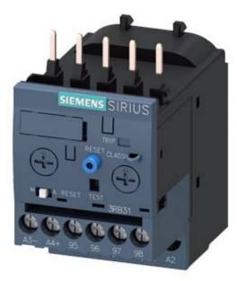
OVERLOAD RELAY 1...4 A FOR MOTOR PROTECTION SIZE S00, CLASS 5...30 CONTACTOR ASS. MAIN CIRCUIT: SCREW CONN. AUX.CIRCUIT: SCREW CONN. MANUAL-AUTOM.-RESET INT. GROUND FAULT DETECTION
