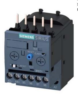
OVERLOAD RELAY 0.32...1.25 A FOR MOTOR PROTECTION SIZE S00. CLASS 5...30 CONTACTOR ASS. MAIN CIRCUIT: SCREW CONN. AUX.CIRCUIT: SCREW CONN. MANUAL-AUTOM.-RESET INT. GROUND FAULT DETECTION
