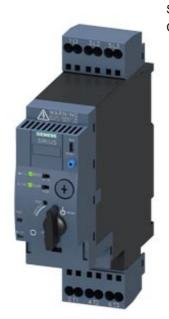
SIRIUS, COMPACT STARTER, DIRECT STARTER 690 V, 24 V AC/DC, 50 ... 60 HZ, 1 ... 4 A, IP20, CONNECTION MAIN CIRCUIT: SPRING-LOADED TERMINAL, CONNECTION AUXILIARY CIRCUIT: PLUGGABLE, WITHOUT TERMINALS
