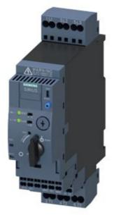
SIRIUS, COMPACT STARTER, DIRECT STARTER 690 V, 24 V AC/DC, 50 ... 60 HZ, 0.32 ... 1.25 A, IP20, CONNECTION MAIN CIRCUIT: SPRING-LOADED TERMINAL, CONNECTION AUXILIARY CIRCUIT: SPRING-LOADED TERMINAL
