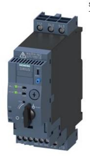
SIRIUS, COMPACT STARTER, DIRECT STARTER 690 V, 24 V AC/DC, 50 ... 60 HZ, 3 ... 12 A, IP20, CONNECTION MAIN CIRCUIT: SCREW TERMINAL, CONNECTION AUXILIARY CIRCUIT: SCREW TERMINAL
