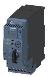
SIRIUS, COMPACT STARTER, DIRECT STARTER 690 V, 110 ... 240 V AC/DC, 50 ... 60 HZ, 1 ... 4 A, IP20, CONNECTION MAIN CIRCUIT: PLUGGABLE, WITHOUT TERMINALS, CONNECTION AUXILIARY CIRCUIT: SCREW TERMINAL
