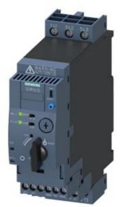
SIRIUS, COMPACT STARTER, DIRECT STARTER 690 V, 24 V AC/DC, 50 ... 60 HZ, 0.1 ... 0.4 A, IP20, CONNECTION MAIN CIRCUIT: SCREW TERMINAL, CONNECTION AUXILIARY CIRCUIT: SCREW TERMINAL
