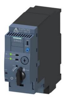
SIRIUS, COMPACT STARTER, DIRECT STARTER 690 V, 24 V AC/DC, 50 ... 60 HZ, 1 ... 4 A, IP20, CONNECTION MAIN CIRCUIT: PLUGGABLE, WITHOUT TERMINALS, CONNECTION AUXILIARY CIRCUIT: PLUGGABLE, WITHOUT TERMINALS
