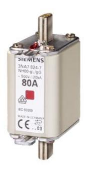
LV HRC FUSE LINK GL/GG WITH NON-INSULATED GRIP LUGS WITH COMBINATION INDICATOR SIZE 00, 125A, AC 500V/DC 250V
