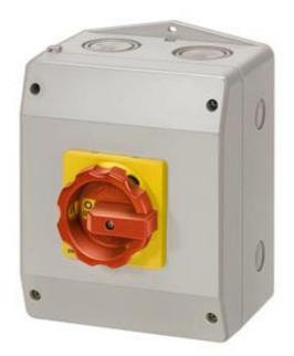
EMERG. STOP SWITCH 6-POLE IU=32, P/AC-23A AT 400V=11.5KW 1NO+1NC, 1 N-TERMINAL INSULATION-ENCLOSED, IP65 ROTARY ACTUATOR RED/YELLOW (EMERG. STOP)
