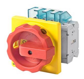
EMERG. STOP SWITCH 3-POLE IU=25, P/AC-23A AT 400V=9.5KW 1NO+1NC, FRONT MOUNTING FOUR-HOLE MOUNTING ROTARY ACTUATOR RED/YELLOW (EMERG. STOP)
