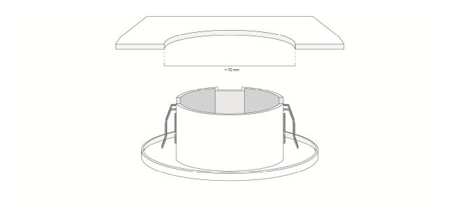
suspended ceiling: dimensions mounting hole diameter
