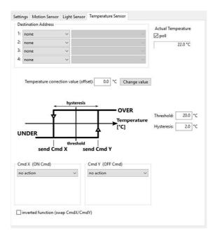
The settings of the temperature sensor are independent from motion and light, another destination address can be used.
