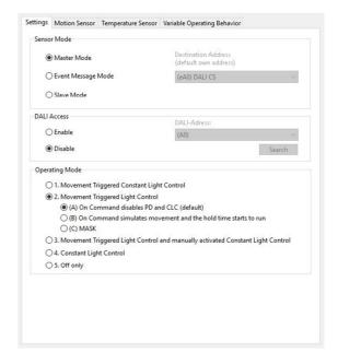
The basic use case of the sensor can be configured with the help of the "Sensor Mode". The module can act either as controller or as sensor unit (e.g. in combination with a central control unit).
