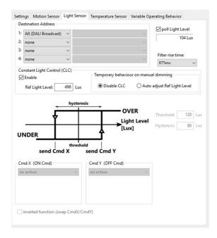
As alternative to the constant light control the light sensor can be used as threshold switch with hysteresis (Threshold (0...1020 lux, Stepsize 4lux), Hysteresis (0...255 lux)).
