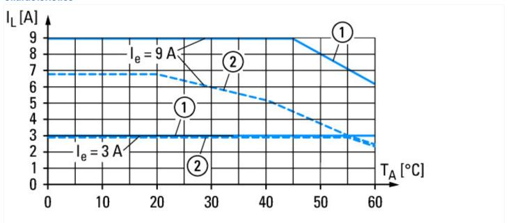
Electricity derating devices with EMS2-XTH adapter
