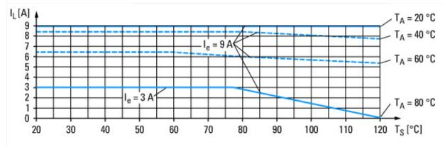
Electricity derating devices with EMS2-XBB or MSFS adapter Devices with  $\rm I_e=9~A$  that are installed with a minimum clearance of 20 mm.
