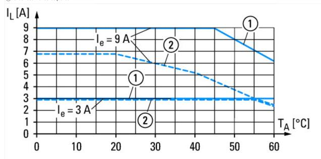
Electricity derating devices with EMS2-XTH adapter
