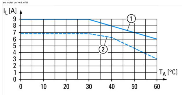
Electricity derating devices with  $I_e = 9 A$
