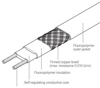
$1.4~\text{mm}^2$  nickel plated copper conductors (10 and 15QTVR2-CT)  $2.3~\text{mm}^2$  nickel plated copper conductors (20QTVR2-CT)
