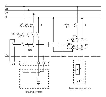
Two- or four-pole electrical protection by circuit-breaker may be needed for local circumstances, standards and regulations \*
