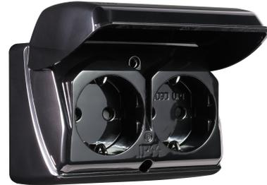
**Product description:** Black AS1090 double earthed socket outlet with hinged cover and child protection. Remember to open drainage hole with fixing. The socket outlet must be installed with the hinges in the top. Classification: IP44 (The lowest IP degree must be considered when combinations of plug and socket outlets are in use)
